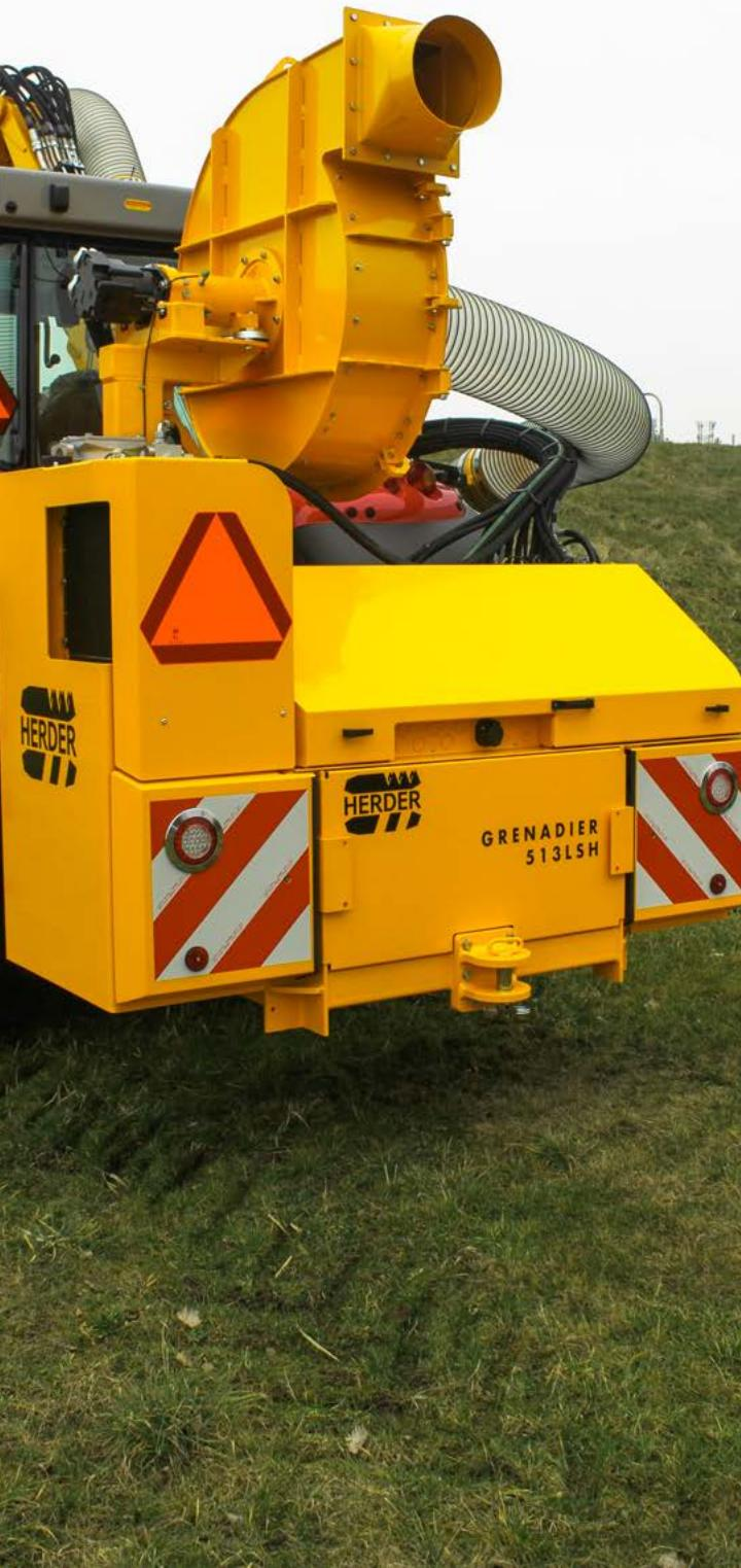
You can also have your Grenadier equipped with an exhaust fan to discharge the cut grass to an attached collection truck. Herder supplies high-quality suction hoses that meet all requirements and have an acceptable lifespan under normal operating conditions. The suction system is easy to maintain due to the easy-to-open fan housing and the detachable suction hose. The hose is available in ø 300 mm.
