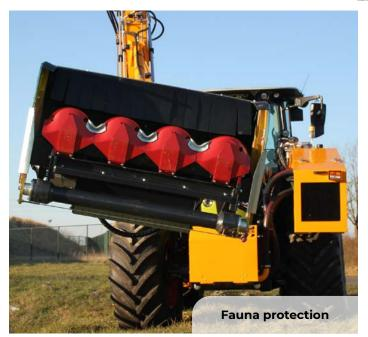
Fauna protection at the mower discs ensures that small mammals, amphibians and insects living on the ground do not get into the mower. Many insects want to jump away when threatened and end up in the discs. The protection plate prevents them from getting into the mower.
