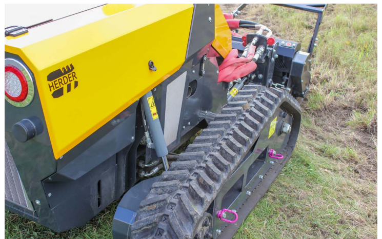
Hydraulic pendulum / adjustment cylinder
