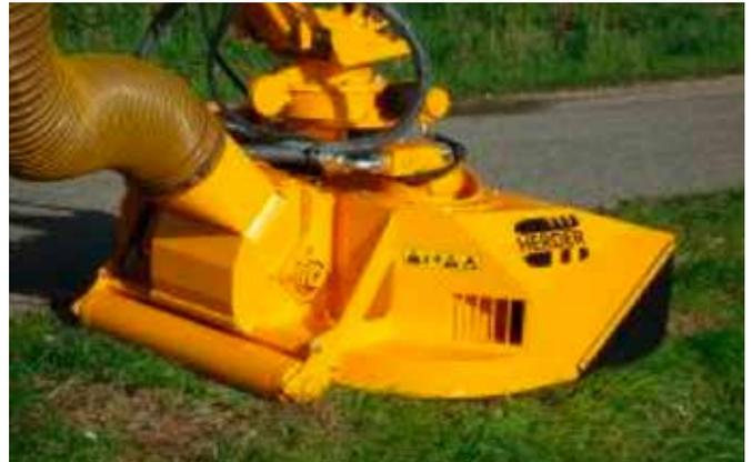
The Herder ecological mower was developed specially and is eminently suitable if you have an ecological mowing policy. The carefully considered construction and design ensure that you can mow in an environmentally correct way. The plant seeds on the ground between the grass and the roots are spared fully. Of course, the same applies to the small animals that live there. If you select Herder's ecological mower, you help take care of preserving the diversity of the roadside.
