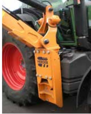
*Pivot 'rotating cylinder' for narrow mounting.*
