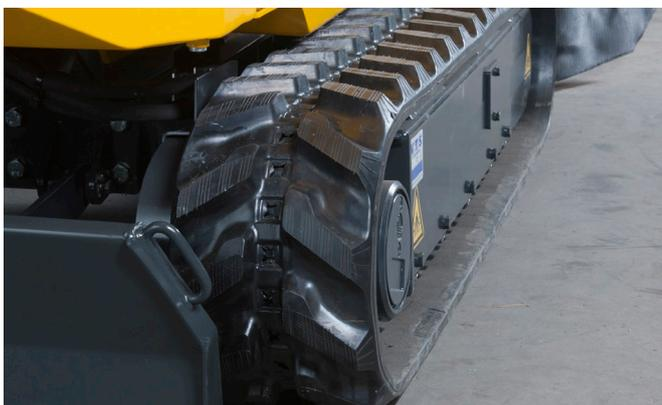
These machines are available on caterpillar tracks, or on a caterpillar undercarriage or 4-wheel model. The SCW-550H and SCW-630H models with wheels (Stump Cutter Wheeled) are supplied as standard with dual tires for extra stability and 4-wheel drive for better driving characteristics on all types of terrain. The dual tires can be removed easily, realizing a width of 85 cm for access to narrow passageways.
